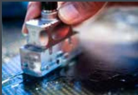
Testing masts, or any carbon laminate structure, is normally undertaken using advanced high frequency ultrasonic techniques. Whilst these may be varied, the use of the medically developed “Phased Array” technology leads the way in providing rapid high resolution inspection. Like medical “Ultrasound,” Phased Array technology produces a highly visual image of the internal structure of the component.
