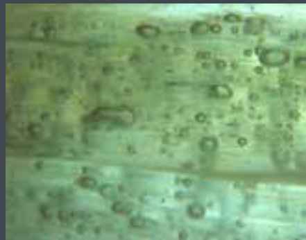
Poor composite construction, porosity in the resin matrix
