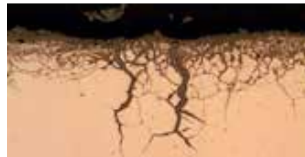
Surface changes and associated cracking
