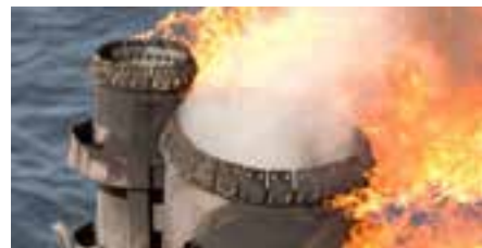
Gas burning around, not inside the flares
