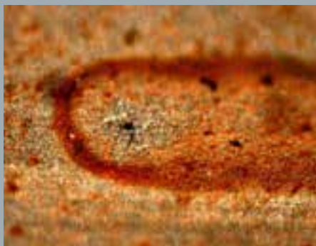
Pinhole corrosion pit inside a pipe
