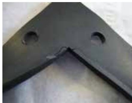
Cracks in the gasket edges
