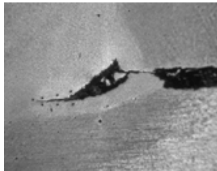
Defective weld cross section
